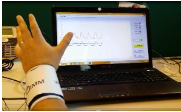
Bracelet for hand/wrist postures and force estimation
